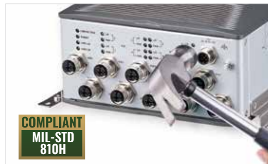
Ultra-rugged enclosure, comply with MIL-STD-810H against vibration and shock impact
