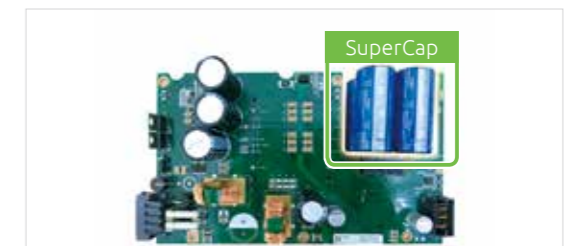
Protection for voltage dips
