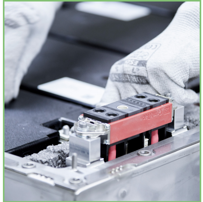
CombiTac connector system carries current and data signals
