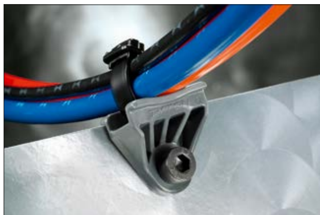
Axial oval mounts stand off bundles from frame rails and cross members to prevent them from rubbing and chafing.
