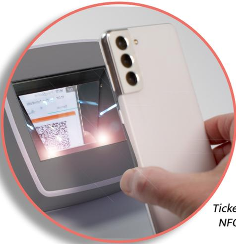
*Ticket readers should support NFC/RFID tickets that can be read in any orientation*
