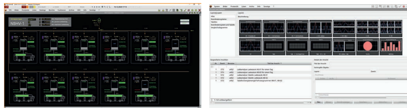
In the event of imminent overload or restrictions in energy supply, power is automatically redistributed to stabilize the grid.
