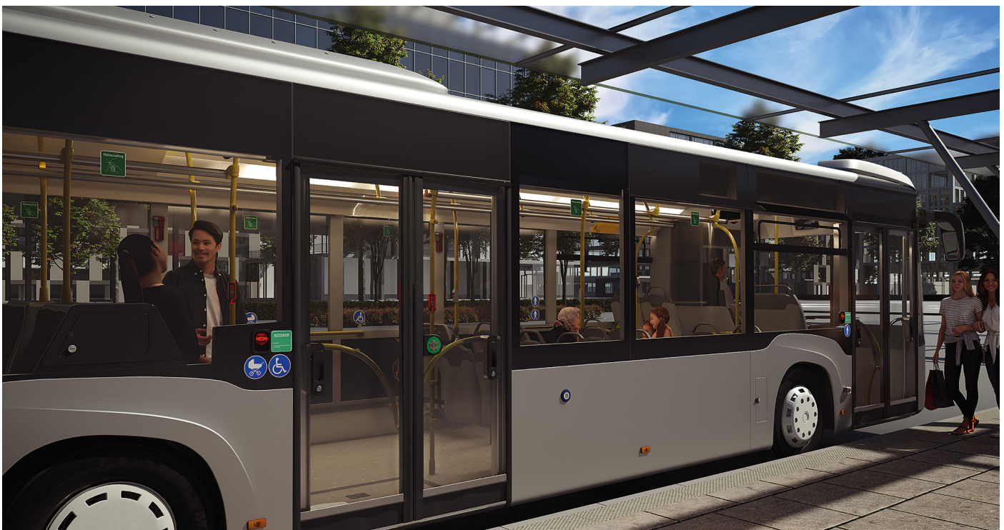
Push buttons in the door area on the outside of the bus help passengers open the doors and meet the normative requirements for handicapped passengers (Photo: TSL-ESCHA)
