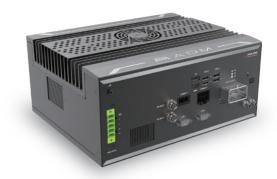
The brains and brawn of this computer are the Intel "Alder Lake-S" 12th Gen i7/i9 CPU and NVIDIA'S RTX 4000 SFF GPU. Intel's 12th Gen chip plays a key role for AV designs owing to its <a href="https://hybrid.processor.microarchitecture">hybrid processor.microarchitecture</a>. Employing distinct, multithreaded Performance-cores and Efficient-cores allows
