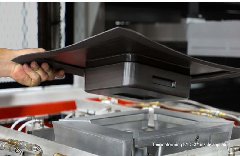
Thermoforming KYDEX® inside appLab™
