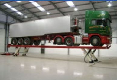
Completely vertical lifting operation
