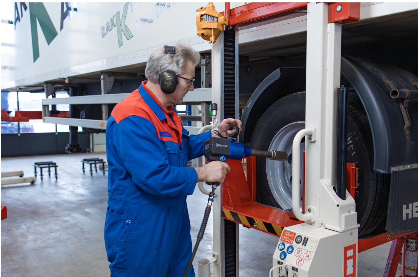
The WD-5P for single, super single and double tyres and wheel combinations from 800 to 1,200mm, and up to 500kg
