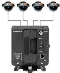
Stand-alone recorder with built-in CAN data recording
