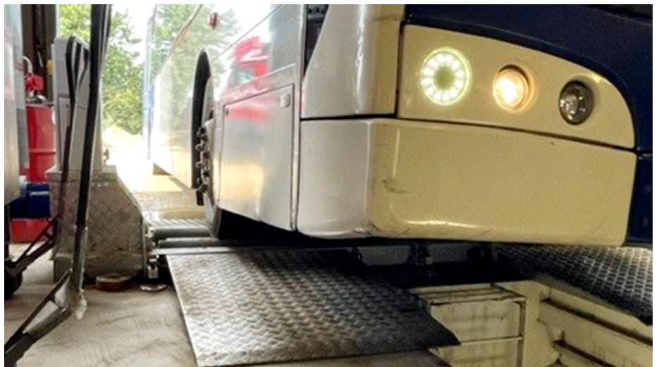
Totalkare mobile brake tester in use at G & C A Lombardo
