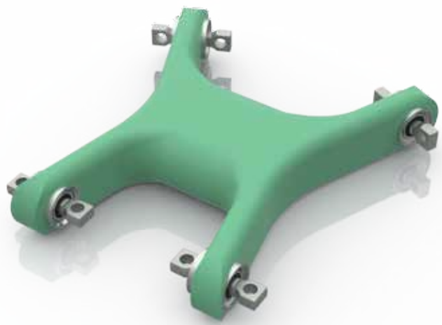
4-point link study using glasfiber-reinforced plastic composite
