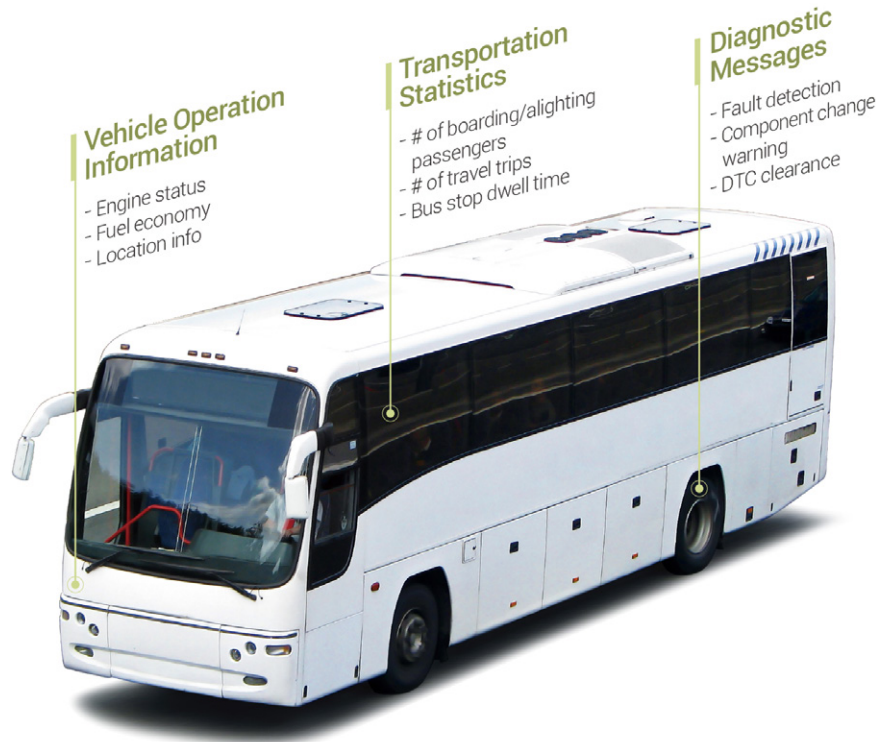
Figure 1. Smart buses are data treasure troves containing vehicle operation information, diagnostic messages, and transportation statistics
