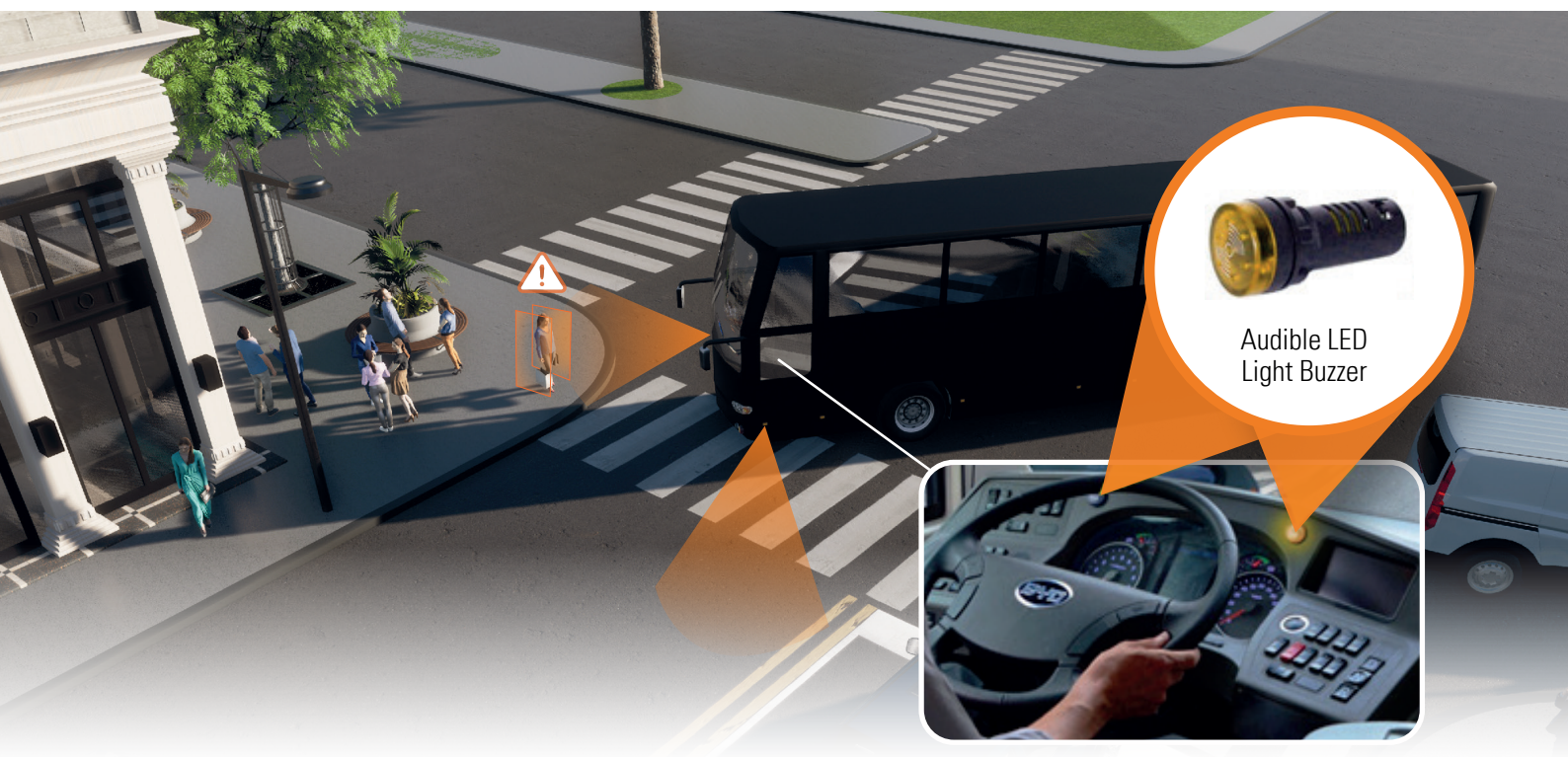
Figure 4. Schematic showing the BSA warning lights on the bus instrumentation panel
