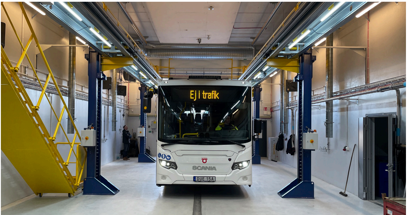
Bus access platforms from Pfaff Verkehrstechnik facilitate maintenance and servicing work on buses
