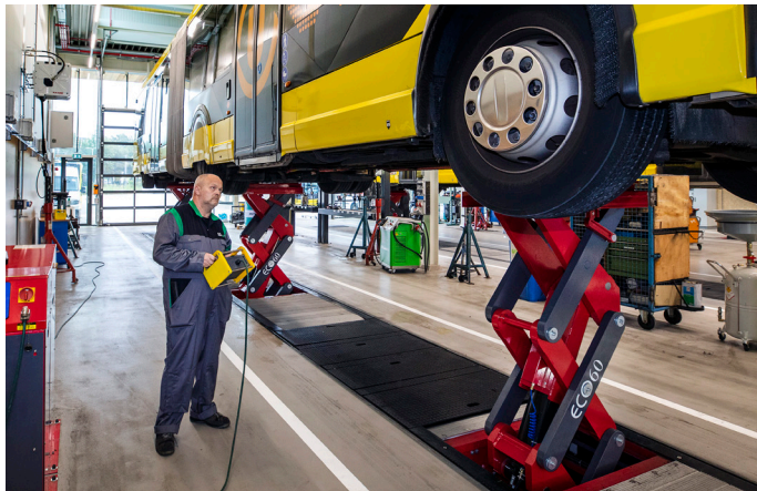
Stertil-Koni in-ground lifts are designed to accommodate vehicles with extremely low ground clearances, such as city transit and articulated buses
