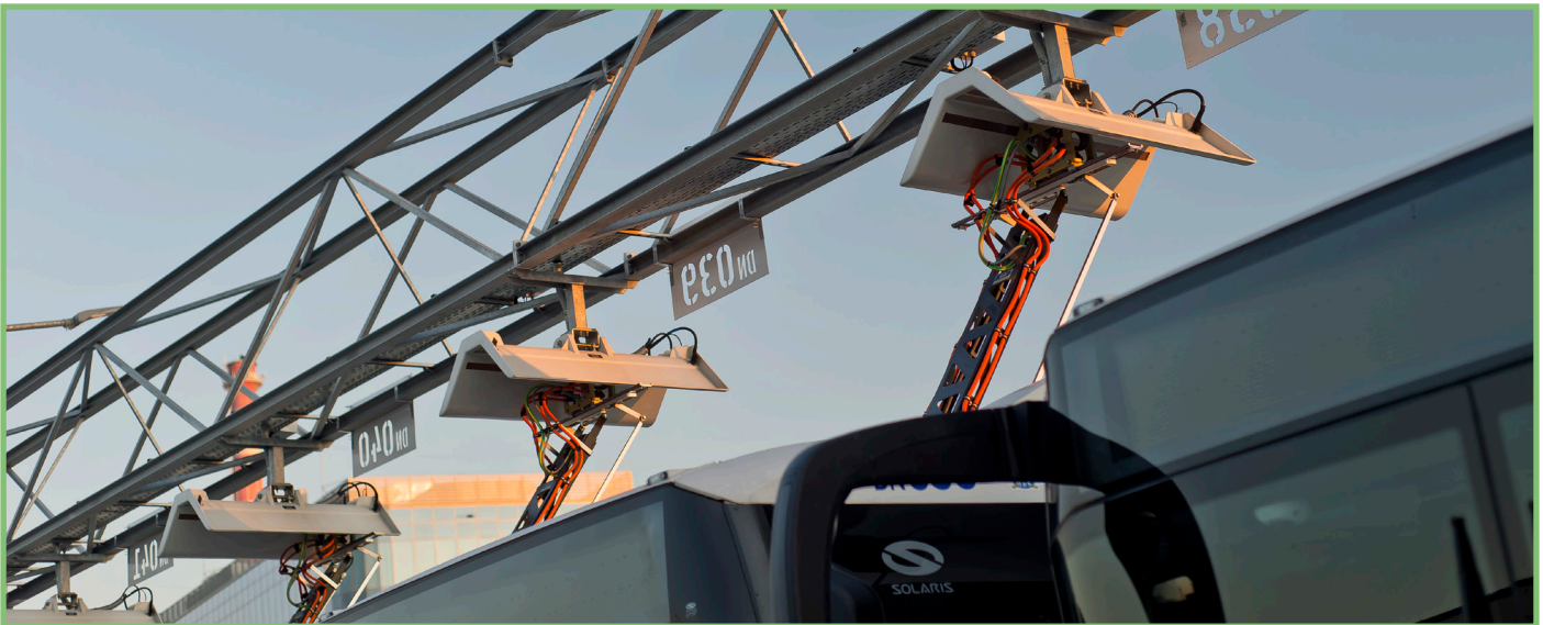
Electric buses equipped with roof-mounted pantographs stop under the charging station where the pantograph extends, connects to the charging station and charges the batteries
