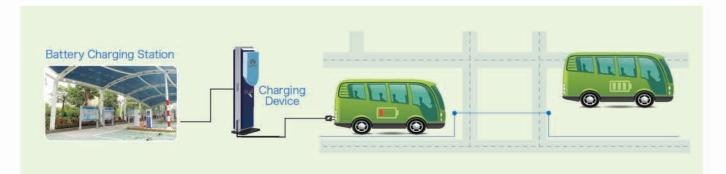
Advantages: : Easy to use, but the charging station needs comparatively small capital investment. Disadvantages:Long charging time and the low efficiency of the charging devices and vehicles. The charging station will need a large construction area.
