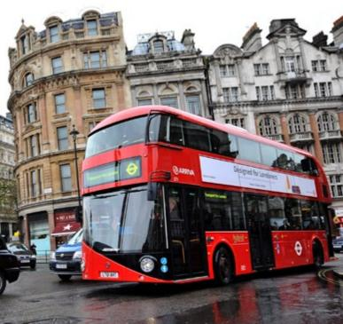
In London, hybrid electric double-decker buses equipped with IPT<sup>®</sup> Charge run in electric mode for more than 80% of the time over an operational day (20h), 7 days a week. Buses are equipped with 60 kWh batteries, and distance between charging options is 11 km.
