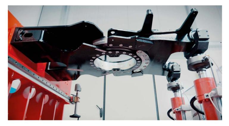
We can thus assess the strength and fatigue states of the materials and the reliability of the components over time.
