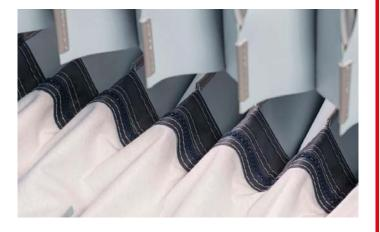
The connecting clips between bellows.
