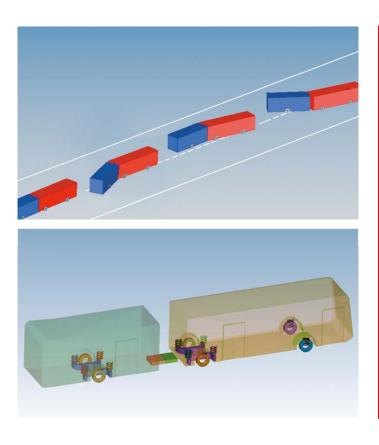
Making use of dynamic simulation software and thanks to great vocation for technological development, PEI Mobility is able to adjust each damping device according to the structure of the vehicle it will serve.
