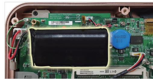
Back-up battery provides uninterrupted power
