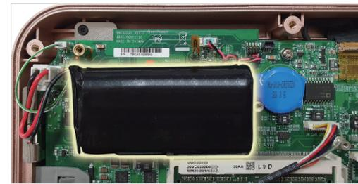
Back-up battery provides uninterrupted power
